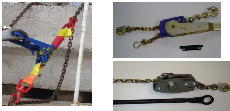
Figure 10: Winch chain tensioners: Left – Web-dog; Top Right: Ausbinder; Bottom Right - EV-Cam (Worksafe Victoria 2010)
