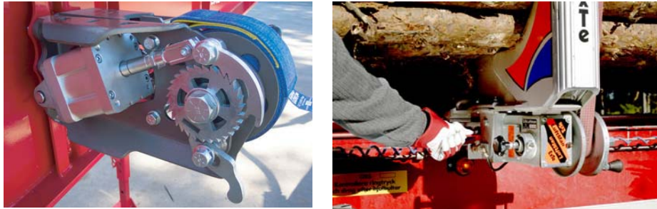
Figure 8. Advanced webbing winches: Elphinstone (left)(Elphinstone 2012); Luftman EXTE (right)(Forest Centre 2012)
