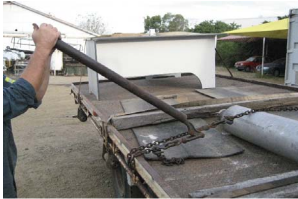
Figure 4. Worker using a dog and cheater bar (Photographer: S. Davis)
