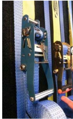
Figure 5: Two types of hand webbing winches (Photographer: J. Chellew)
